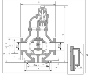
Jacket cover for heating or cooling Maximum pressure 14 bar
