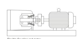
Flexible Coupling and motor.
