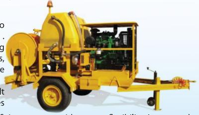
(150mm to 1,000mm bore) in a fast and efficient manner with greater flexibility. It rotates the hose, allowing the nozzle to jet the high pressure water around the internal surface of the pipe. The feed unit will feed or pull the hose automatically in or out of the pipe.
