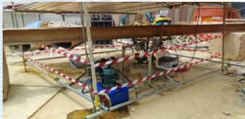
Catholic High School, Singapore (800mm dia, 6.12 MN load, 1,000 mm dia, 5.72 MN load, year 2014)
