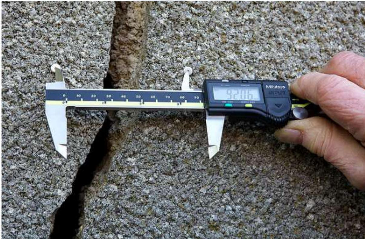
Fine Resolution Monitoring can be achieved using high precision calipers to measure distance between discs located on either side of the crack.
