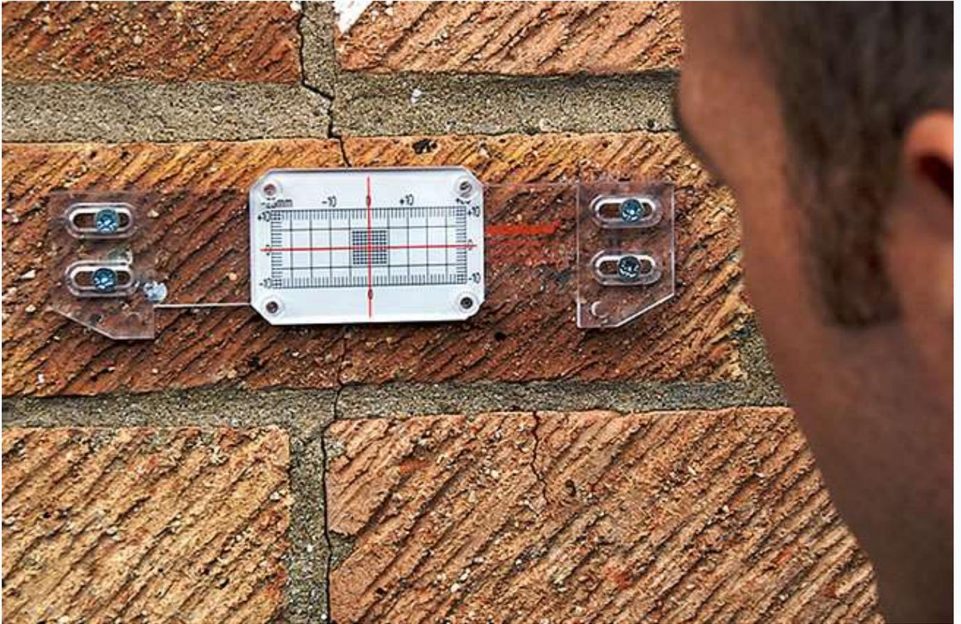
Tell-Tales crack meters are suitable for use on both on internal and external cracks.
