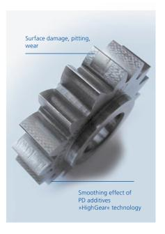
Both mineral oil-based and polyalphaolefin-based products are thus available which fulfill the highest technical standards. The results of tests performed in extreme conditions and with pre-damaged machine elements in large-scale gearboxes (in underground mine conveyor drives) as well as spindle drives in forging presses confirm these outstanding characteristics.
