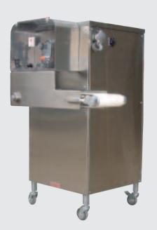
This machine is designed to divide Arabic and Pies dough. It is equipped with a special compressor (Spiral) to push the dough. It cuts the dough in sizes varying between 40 to 200 grams. The body is made of solid metal and covered with stainless steel sheets.
