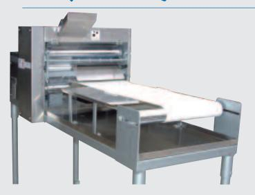
This machine has the required high technique and the accuracy to turn the dough balls into circular loafs having a diameter between 10 and 40 Cm. The external layer is made of stainless steel. Available in various sizes according to the demand.
