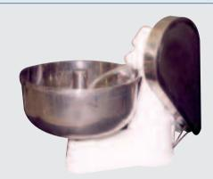
This machine is fabricated to produce different kinds of dough used in the production of Arabic bread and pies. The bowl is made of stainless steel or a rust resistant aluminum. Available in various sizes according to the demand.
