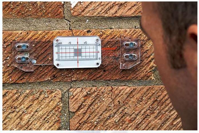
Tell-Tales crack meters are suitable for use on both on internal and external cracks.
