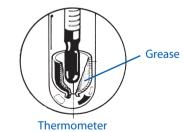
18. Water resistance — Static test as defined by DIN 51807-1
